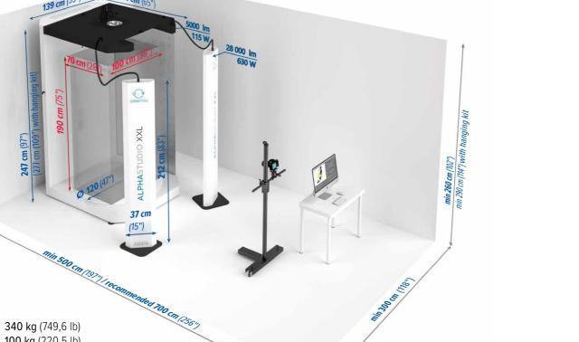
📩 Max load 100 kg (220,5 lb) Power supply 100-230VAC, max. 1495W
